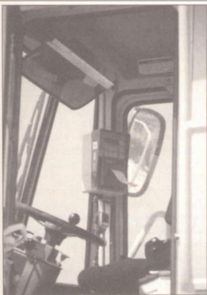
In-cab display and print-out for VEI's weighing system.
