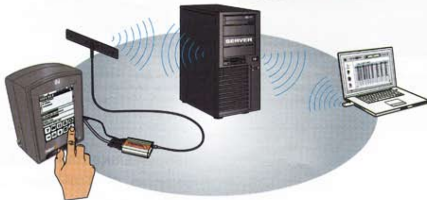
Trackweight sending data to VEI server and collecting data from the internet
