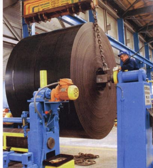
Finished belt being strapped for despatch from Apex Fenner's new plant.
